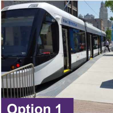
Option 1 Introduce low-floor, level-boarding vehicles—Faster boarding
