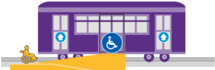
High Platform – Switchback Ramp
